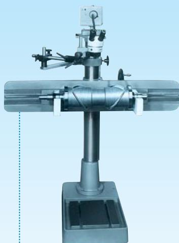
Regrind station to regrind and sharpen the knives. Precision-stereo-microscope with wide angle eye pieces, installed in a swivel mount camera system with monitor available as option.
