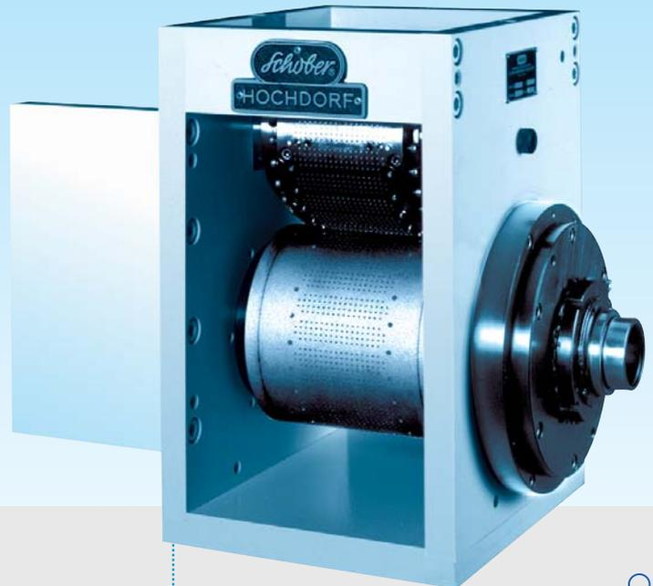
Punching module for band-aid material with hollow die cylinder and exchangeable punches. Even in a dense punching pattern with a whole diameter of 0.9 mm the waste is effectively removed.
