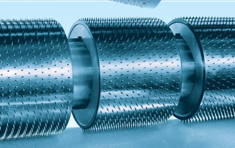
Cylinder with moveable needle rings for hot and cold perforation. Depending on the specific requirements the anvil can be made of rubber or steel.
